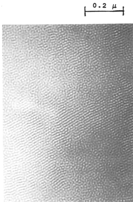
Figure 3. TEM micrograph of the ultrathin cross section of the bulk of a PDMS-PS-PDMS triblock copolymer (sample 8). The period is about 130 Å.
